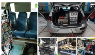
Figure 3. CRMT installations for RDE emission measurements of: (a) bus; (b) car; (c) street sweeper; (d) flow measurement in a truck; (e) PEMS and FTIR.
